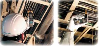
Measurement reading reverses automatically when the display is flipped open to ensure readability.
